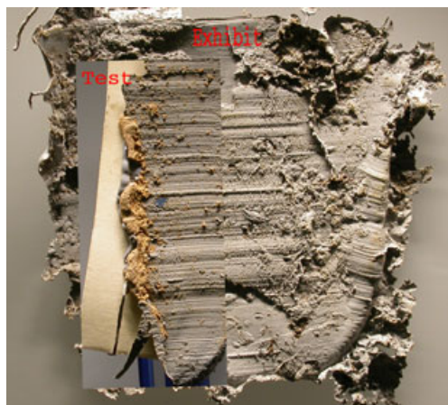
FIG. 8—Digital photograph comparison of cast of marks caused by mattock (insert) to cast of clod of soil.
