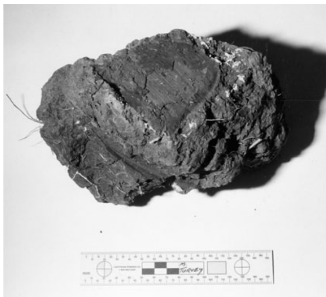
FIG. 1—Clod of soil recovered from gravesite depicting striated toolmarks.
